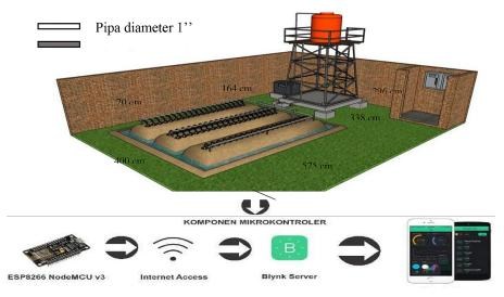
Fig. 1. IoT-based drip irrigation system design
